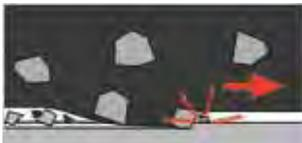
During cutting, the exposed diamonds may crack or break (all the more rapidly, the harder and denser the material)
