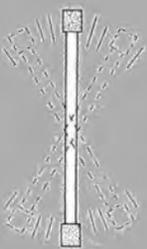
1. Blade retainer on some makes of saws have a 'cupped' shape allowing the reducer ring to offset. Even just a slight offset causes increasing wobble as the RPM's increase.
