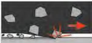
The diamonds exposed in this way cut into the material reducing it to fine powder.
